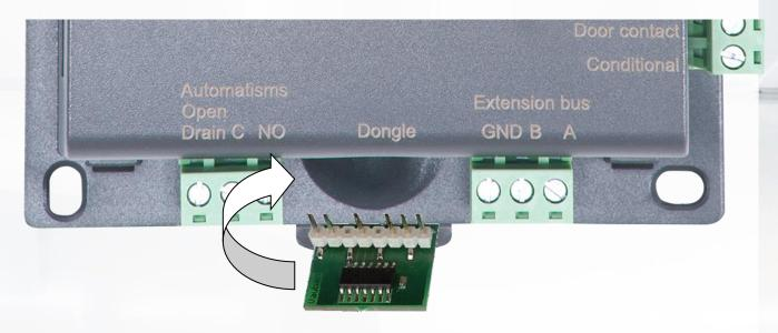
To confirm proper operation, **VISOR** shows the version being used at the bottom of the main screen. Your unit must be rated for the dongle to be detected.
