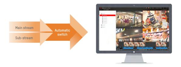
Main stream and sub-stream automatic switching maintains quality resolution for display when multiple cameras are viewed by one client simultaneously thus saving bandwidth while providing monitoring details.
