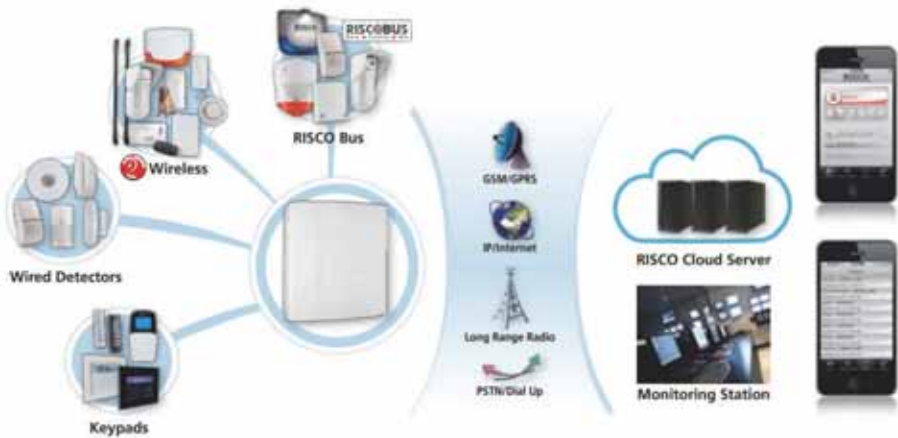
Figure 1-1 Architecture de la LightSYS2
