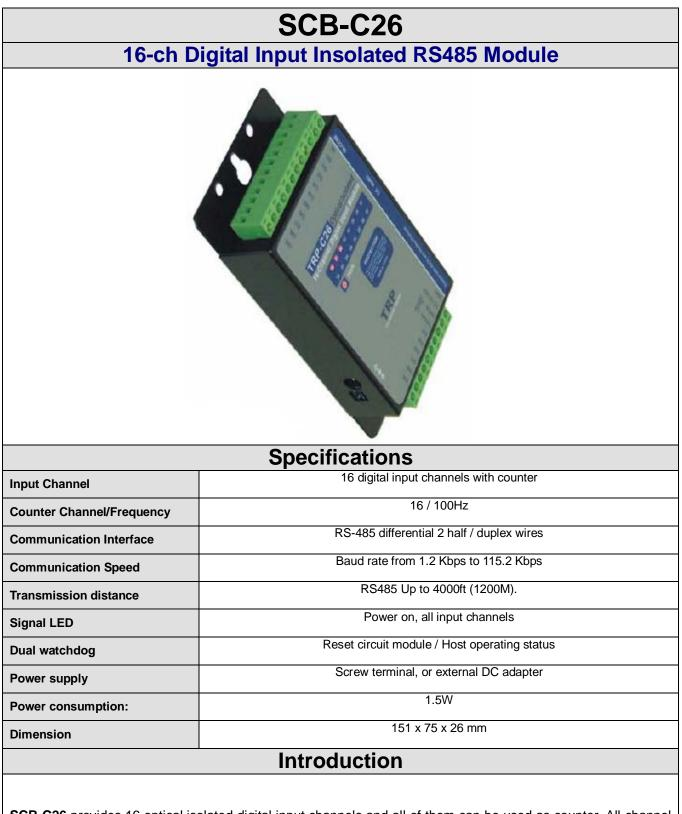
**SCB-C26** provides 16 optical isolated digital input channels and all of them can be used as counter. All channel features screw terminals for convenient connection of field signals as well as LED's to indicate channel status. All inputs are equipped with photo-couplers to protect the module against high voltage spikes and ground potential differences.
