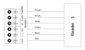
Figure 7 Wiring for Reader 3
