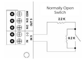
Figure 4 Normally Open Supervised Inputs with Double Resistor
