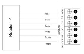
Figure 8 Wiring for Reader 4
