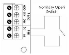
Figure 1 Normally Open Input
