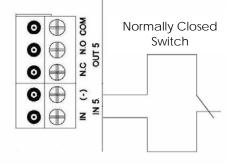
Figure 2 Normally Closed Inputs
